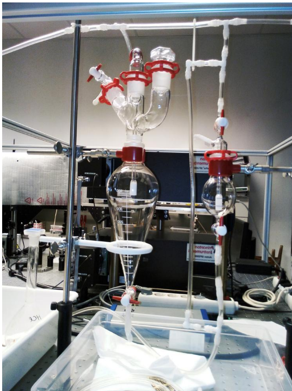
Figure 4.8: Photo of the chemical setup: The gas flow to the containers can be controlled at the top, where the gas outlet is as well. The argon enters the containers through a glass tube and gets dispersed through a porous glass element at the end to create small bubbles, when submerged.
